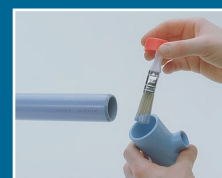
3 - Bonding with welding polymer
